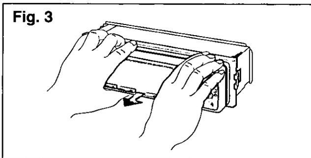
**Note:** Do not lose the Dismounting Plate. It will be needed to remove the unit from the car's dashboard.
