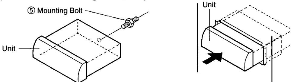
d) Secure the rear of the unit to the car by either of the two recommended methods.
